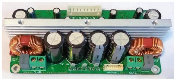
Figure 1: CxD2160 Amplifier Module appearance
