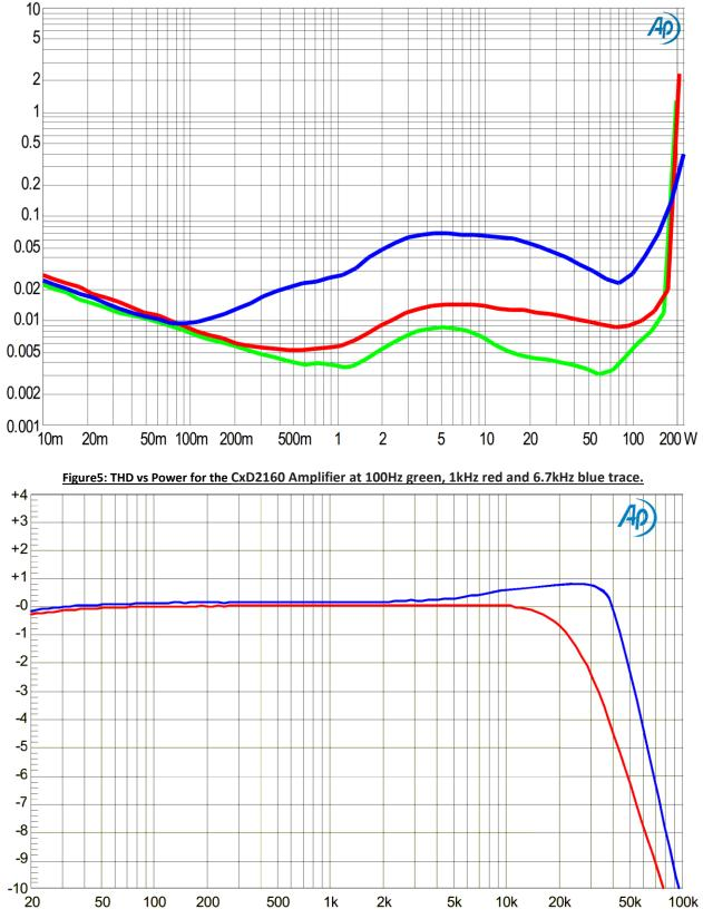
**CxD2160 Amplifier Module measurements and performance:** To characterize the CxD2160 Amplifier Module performances, some relevant measurements were done and displayed below:
