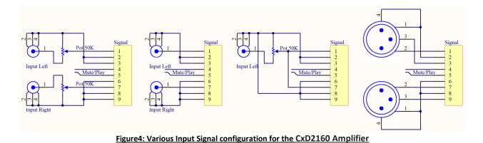
Several input signal connection configurations are possible, four of them are shown in **Figure4** above. For simplification, only the input connector is shown with various input wiring configurations, from left to right:
