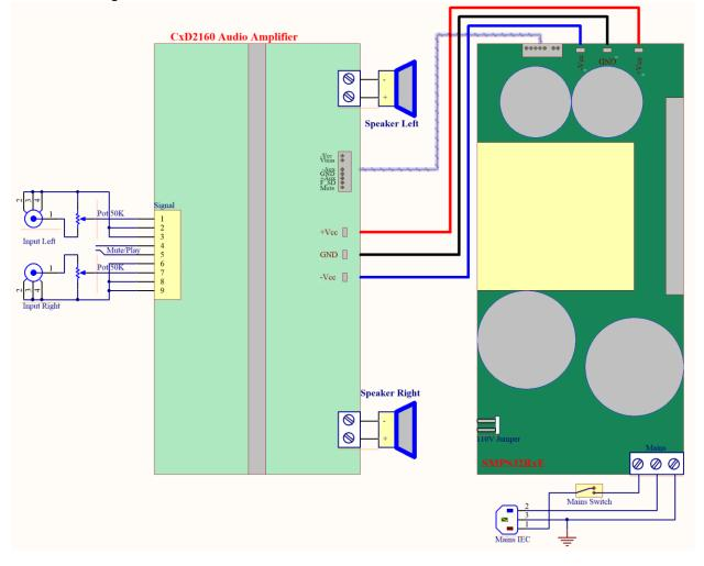
Figure 2: CxD2160 Amplifier Module & SMPS320RxE Interconnection using unbalanced RCA connectors and potentiometer
