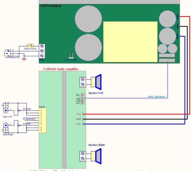
Figure 3: CxD2160 Amplifier Module & SMPS500RxE Interconnection using unbalanced RCA connectors
