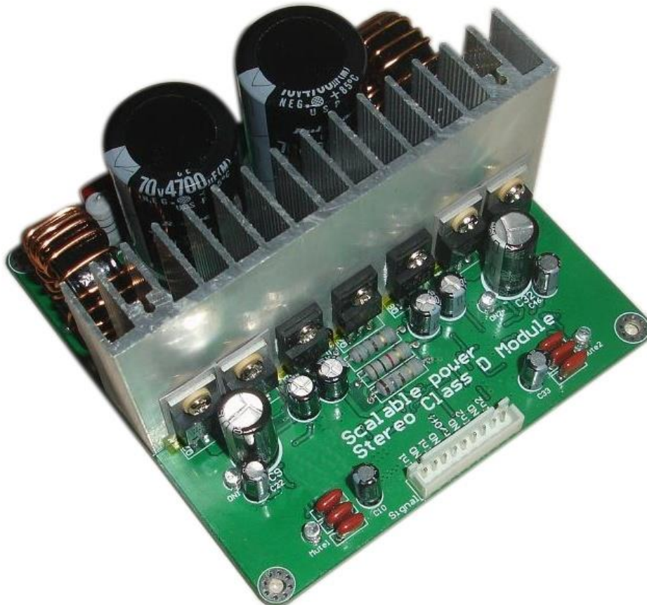
Figure 1: IRS2092 Stereo Audio Amplifier Module
