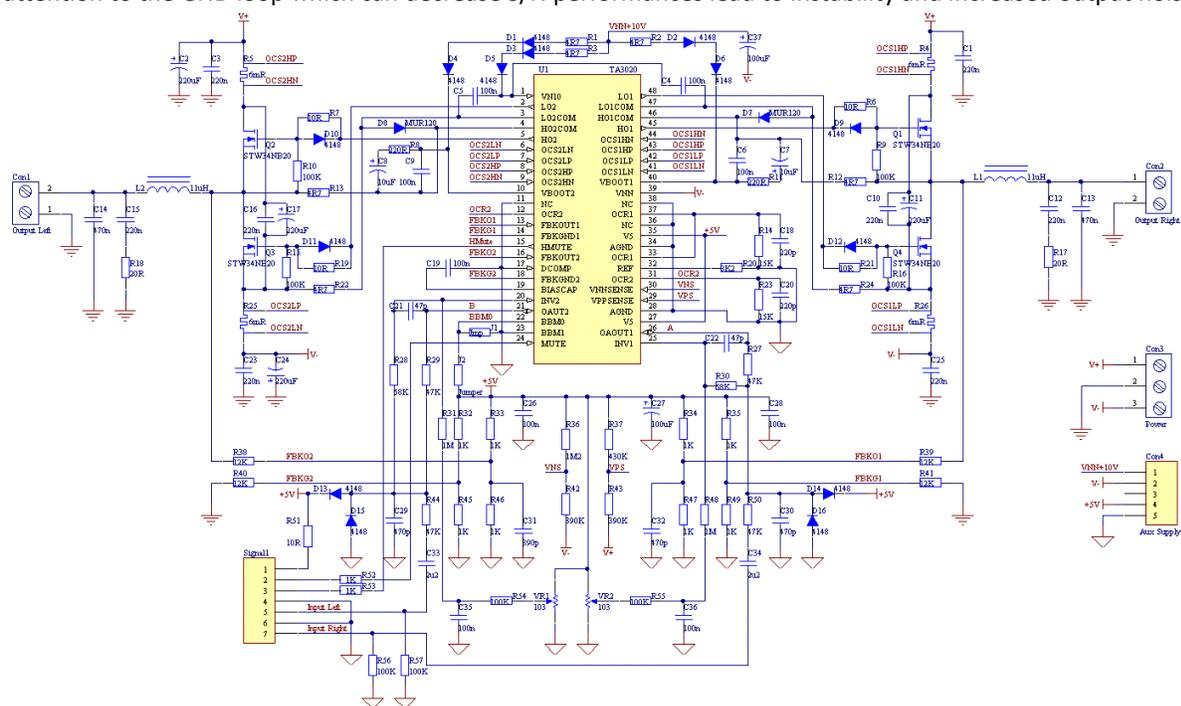
Figure 2: TA3020 v3a Audio Amplifier Module Schematic Diagram
