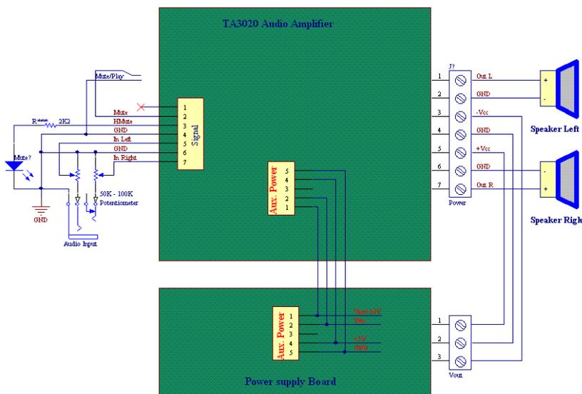
The main differential voltage should be supplied on the connector 3, which is in the top middle of the board, between the output connectors. See the Figure 5 for connectors positions reference.
