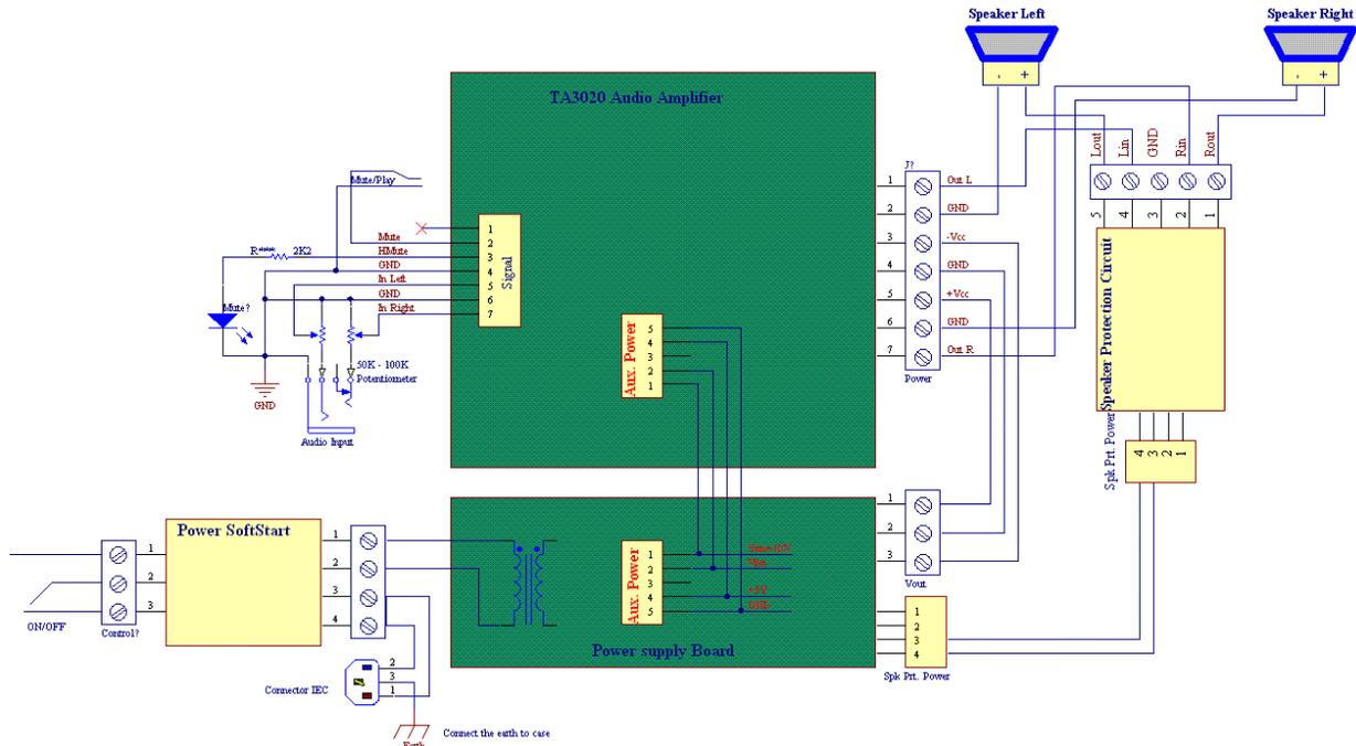
**Figure 5: TA3020 Audio Amplifier Module supply connection diagram with Speaker Protection and PSS modules**
