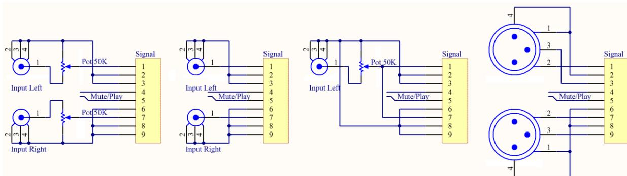
**Figure4: Various Input Signal configuration for the CxD2160 Amplifier**
