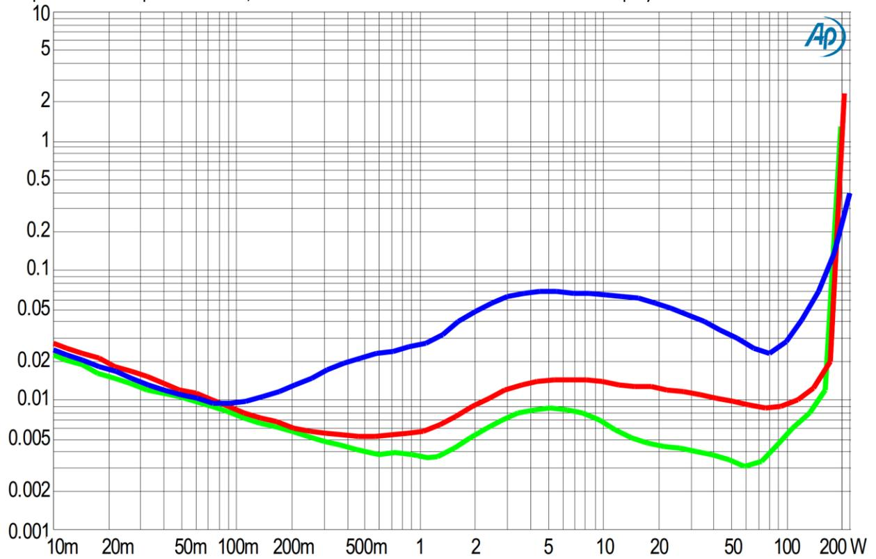
**Figure5: THD vs Power for the CxD2160 Amplifier at 100Hz green, 1kHz red and 6.7kHz blue trace.**
