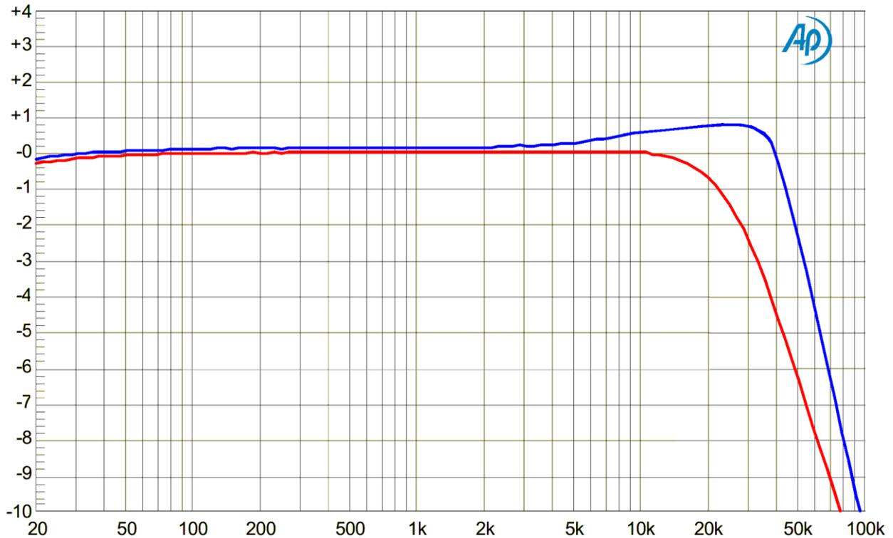
**Figure6: Frequency response of the CxD2160 Amplifier: red trace: 4Ω load impedance blue trace: 8Ω load impedance.**
